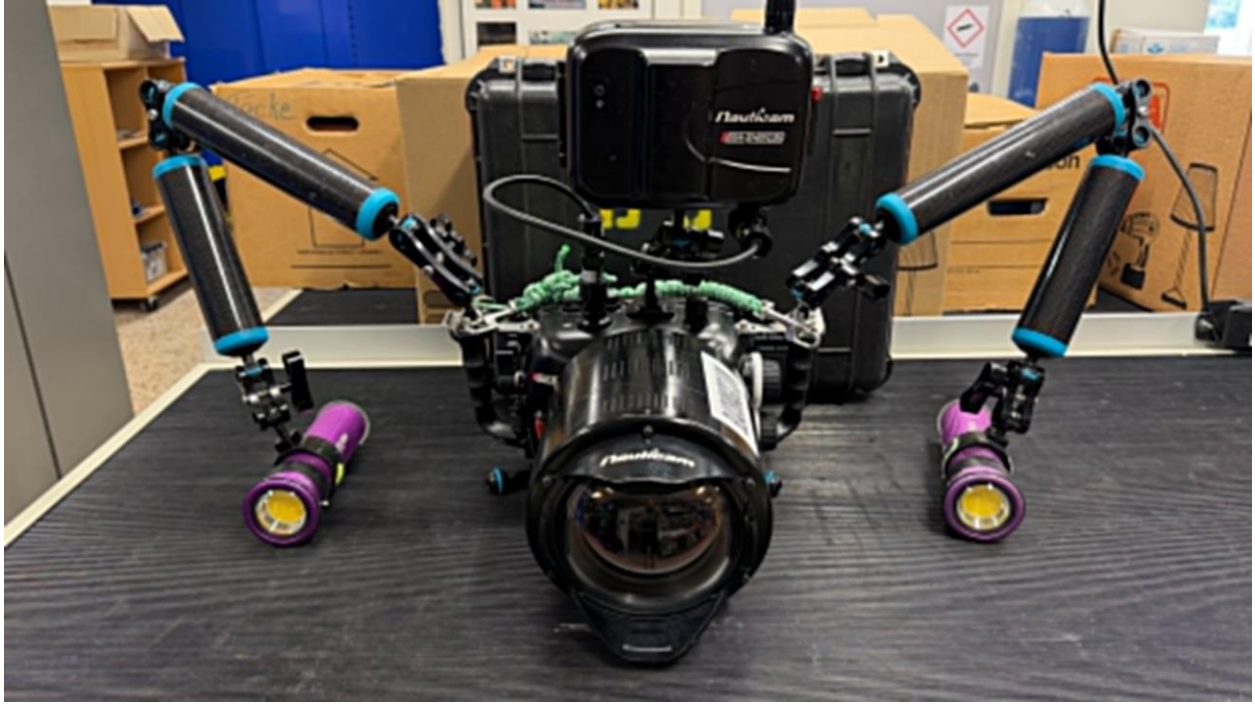
Figure 10 Black Magic 6k camera with Nauticam underwater housing used during the project.
