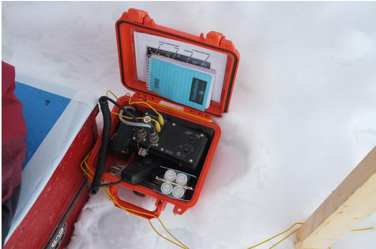
Figure 14 Heyphone in its transport case, yellow wires (max 2x25m) go to both earth antenna connectors (photo Bo Lenander)
