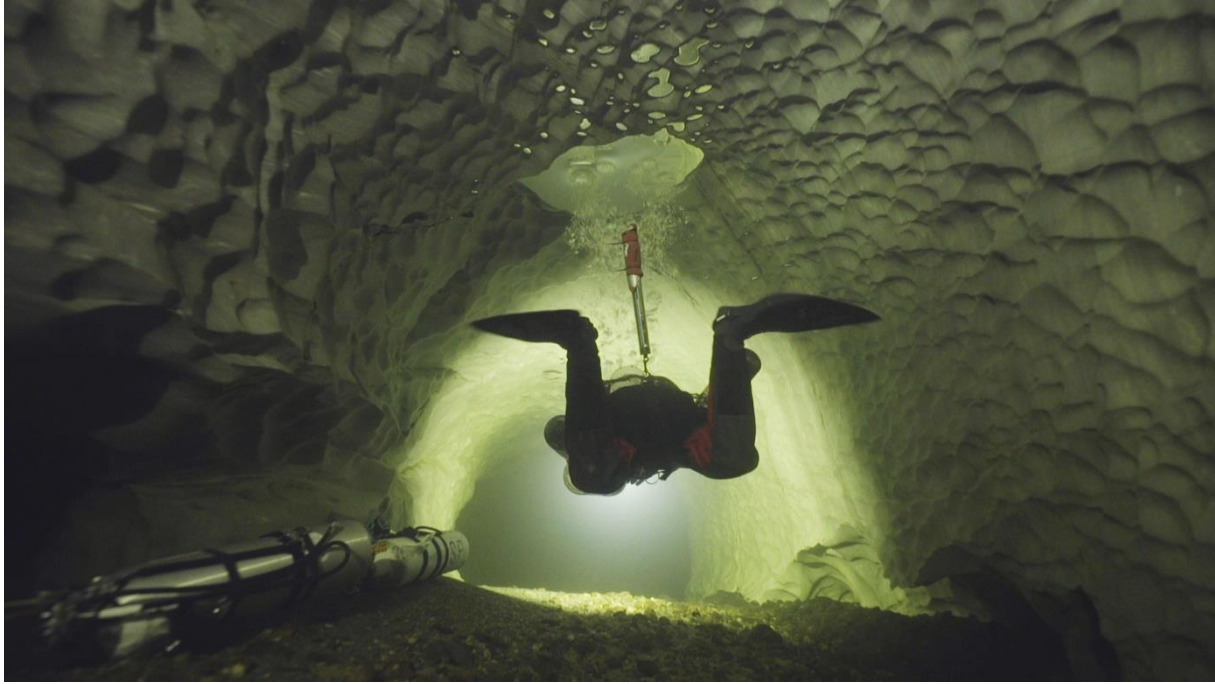
Figure 13 A diver equipped with a M-16MK marker (here attached to the rear d-ring) can be followed and identified from the surface (photo Janne Suhanen)
